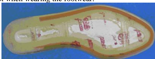
Figure 4: Insole with an elevation made with the help of plastic mass
