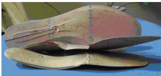
Figure 6: Insole with injected reinforcement with a metallic joint
